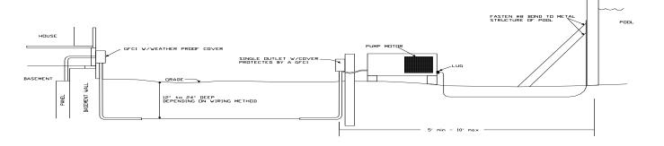
Overhead power lines must be at least 10-feet horizontal from the edge of the pool and 22.5 feet in any direction of the waters edge.
